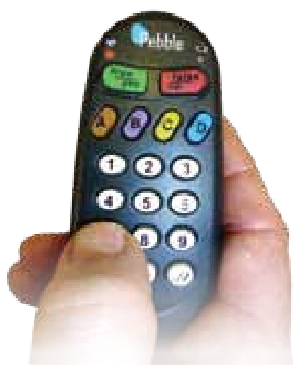
A non-mapped handset will show a red light when any key is pressed.
