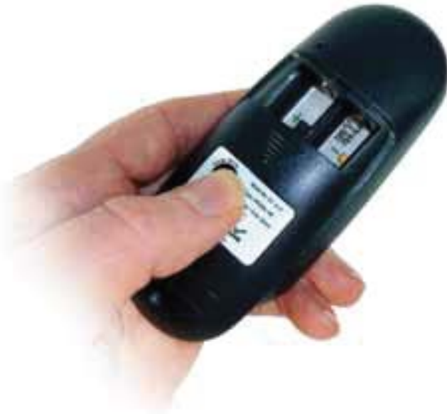
1. Pebble pad battery cover being removed
