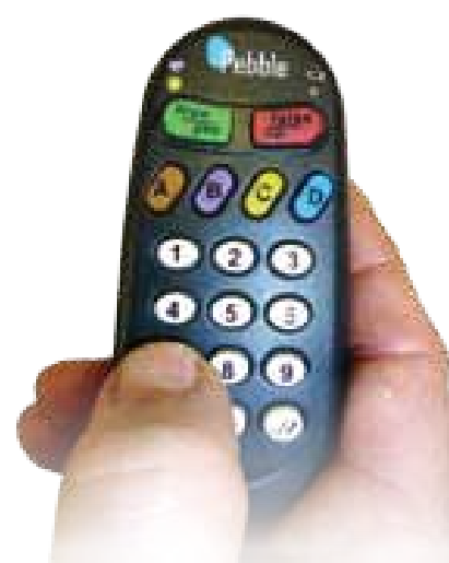
The communication LED will blink GREEN 3 times when mapping is complete.
