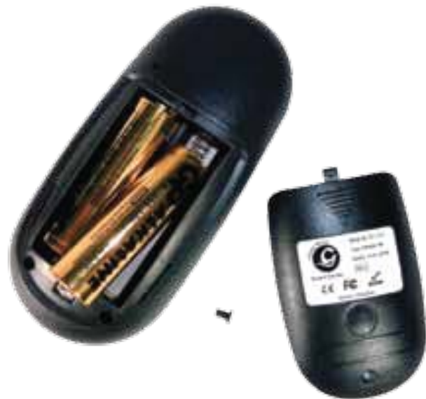
2. Batteries being inserted
