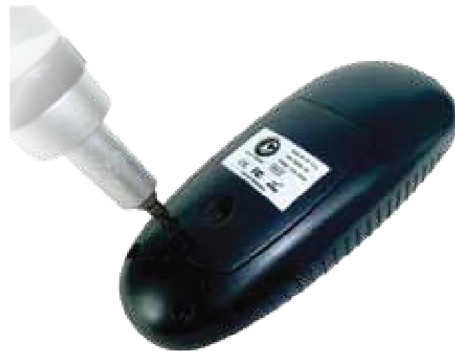
3. Battery cover being screwed on
