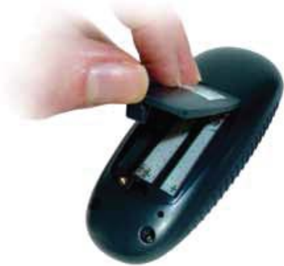
1. iQ-Pad battery cover being removed
