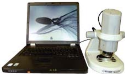
GENEE SCOPE CONNECTED TO LAPTOP USING USB
